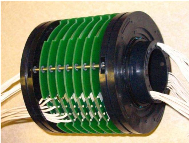
**Figure 6: AC 6815--Broadband platter construction**
