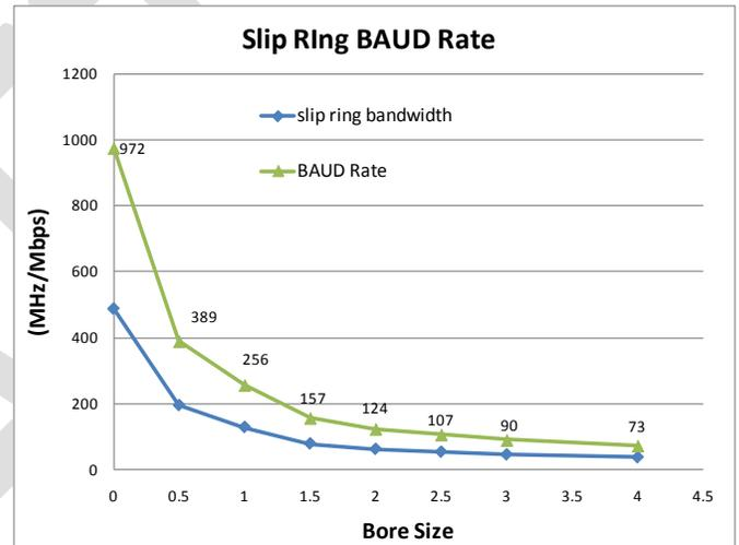
Figure 4: Bandwidth and baud Rate Guidelines for Drum Style Slip Rings
