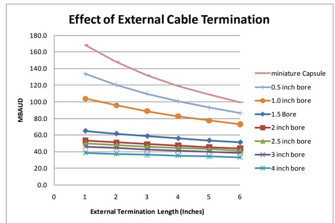
Figure 5: Effect of Cable Termination Outside the Slip Ring Housing
