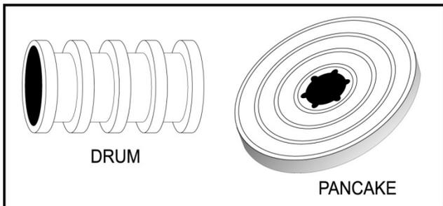
Figure 3: Platter and Drum Style Slip Ring Design
